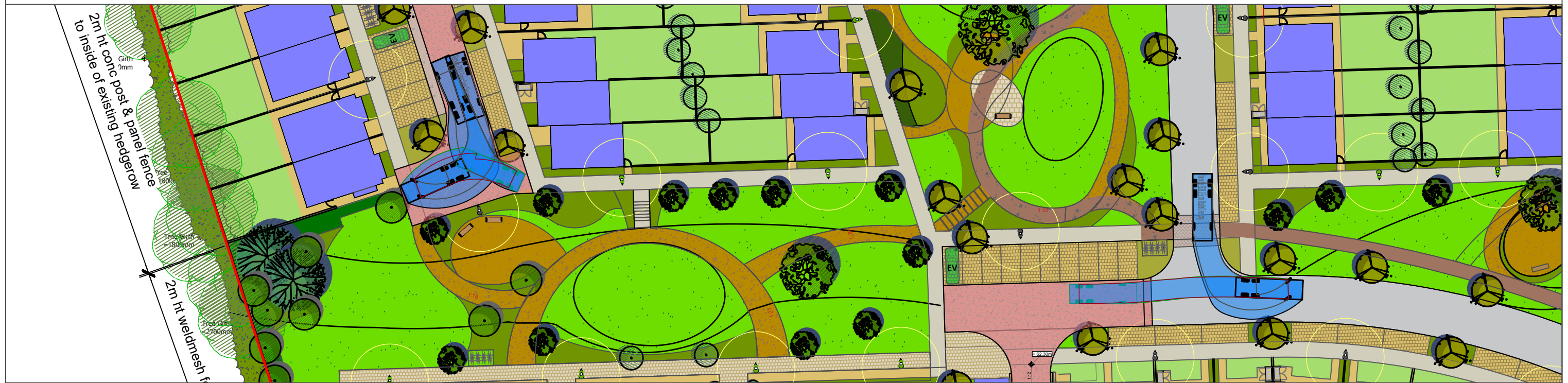
AUTOTRACKS OF 2No. SOUTHERN TURNING HEADS
